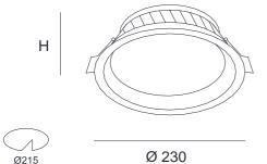
cut-out dimensions: Ø 215 mm recessed depth: 95 mm
