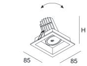
cut-out dimensions: 75x75 mm recessed depth: 120 mm
