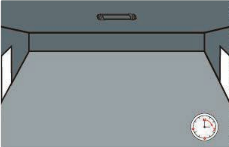
When time-lapse mode ends, the luminaire will turn off if no motion detected.
